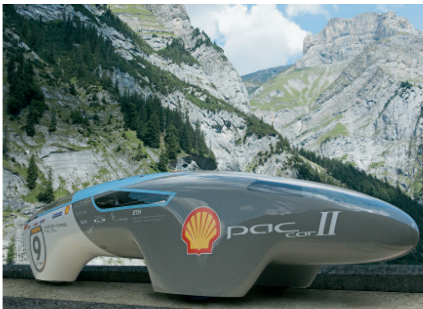
Fig. 1: Demonstrating the latest innovation in automotive engineering, ETH Zurich together with external partners built the most fuel-efficient vehicle in the world. PAC-Car II is equipped with a fuel cell to convert hydrogen into electricity to power its electric motors; it has a range of 5385 km with a hydrogen equivalent of 1 litre of petrol: www.paccar.ethz.ch . Climate KIC: www.climate-kic.org
